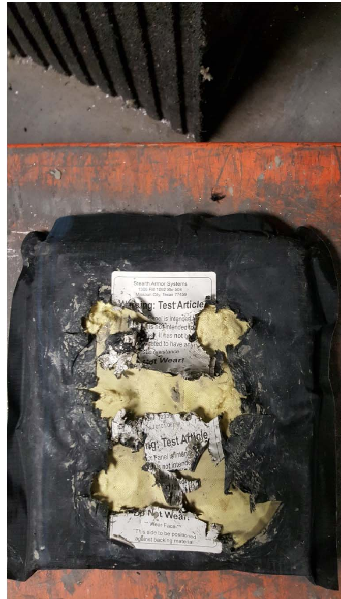
4-P-BFS Plate #1_Body Side_Post-test
