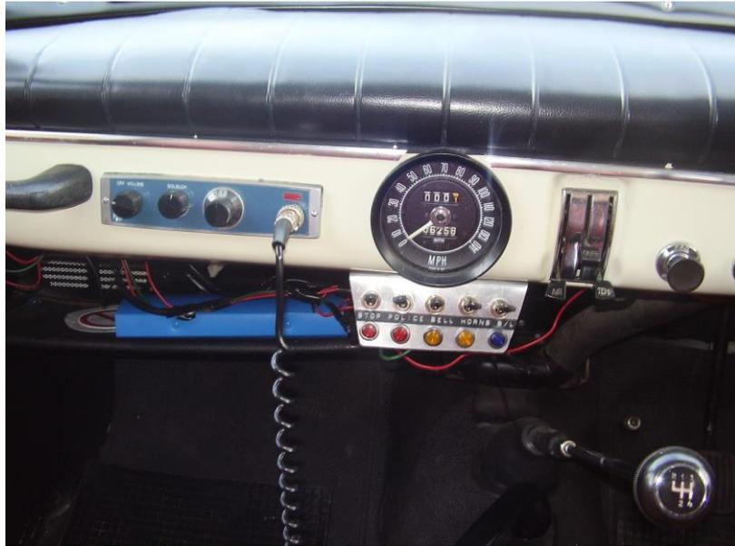
*The new dash panel with Smiths calibrated speedo and all the necessary switch gear*
