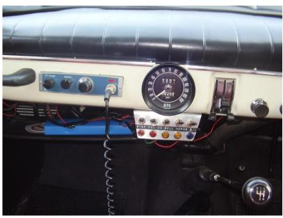
The new dash panel with Smiths calibrated speedo and all the necessary switch gear
