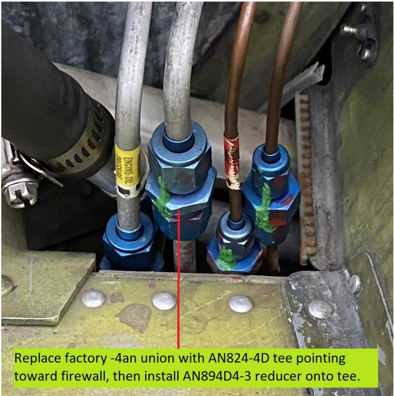
Figure 1-2. Factory Manifold Pressure Union
