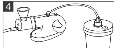
4 Place the other end of the vacuum hose on the suction hole of the vacuum tank, air valve vacuum bag, wine stopper, etc.
