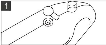
1 Connect the vacuum hose to vacuum adaptor. (use the small port).
