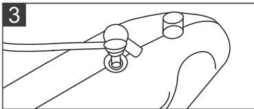
3 Long touch the on/off button for 3 - 5 seconds to start vacuum function, Green light will be flashed.
