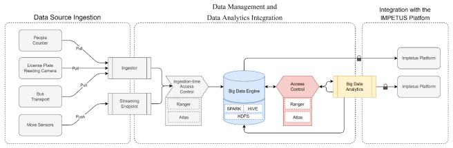
Figure 31: Data management and data analytics integration - Mapping to the Engine
