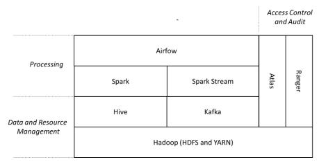
Figure 5: Big Data engine architecture
