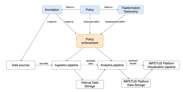
Figure 7: Policy Enforcement within the pipeline execution
