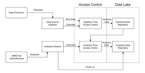
Figure 19: Integrated Big Data platform flow
