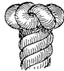
The "Wall Knot" (Fig. 114) is almost as simple as the crown, and in fact is practically a crown reversed.
