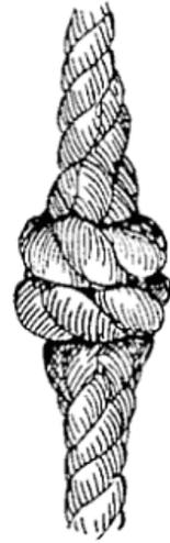
As in the case of the crown knot, the wall is mainly of value as an ending when ends are tucked, or as a basis for more ornamental knots such as the "Wall and Crown," or "Double Wall," or "Double Crown." It is also very largely used in making "Shroud Knots" (Fig. 117).
