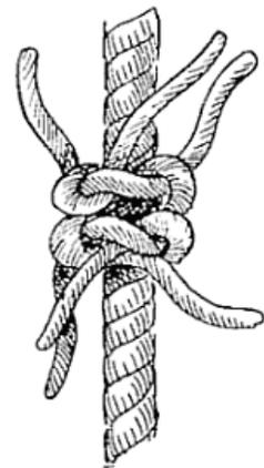
The common shroud knot is made by opening up the strands of a rope's end as for a short splice and placing the two ends together in the same way. Then single "wall" the strands of one rope around the standing part of another against the lay, taper the ends, and tuck and serve all with yarn or marline (Fig. 118).
