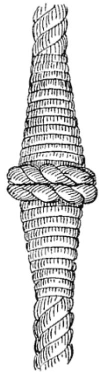
FIG. 120.—French shroud knot (complete).
