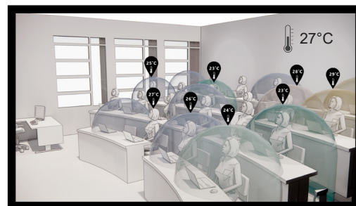
Figure 5: Conductive Cooling_27°C PECS with HVAC System in the classroom
