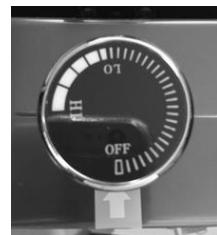
After the cartridge has been loaded, the Adjustment Knob can then be slowly screwed in a clockwise direction until the Pressure Indicator reads the desired amount of flow of the CO<sub>2</sub>. This is known as **engaging**, or **turning ON**, the device.
