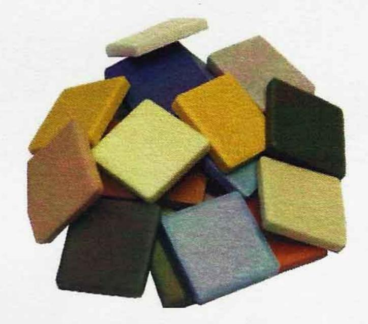
25mm x 25mm x 4mm vitrified porcelain tiles, unglazed but with a soft sheen. Mazurka offers the largest selection of colours in the mosaic palette in this type of tile, from subtle to strikingly vibrant shades. The tiles are frost proof, suitable for interior and exterior use and useable in high traffic areas. Very easy to cut with sidebiters or wheeled tile nippers. Available from Mosaic Supplies in strips of 72 tiles on mesh and as loose mixed colours.
