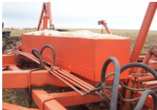
A home made rock box topped with concrete
