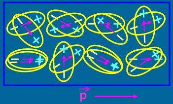
When electric field is applied, the dipoles orient themselves in a regular fashion and hence dipole moment is induced. Complete allignment is not possible due to thermal agitation.
