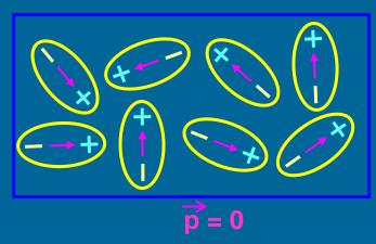
In the absence of external electric field, the permanent dipoles of the molecules orient in random directions and hence the net dipole moment is zero.
