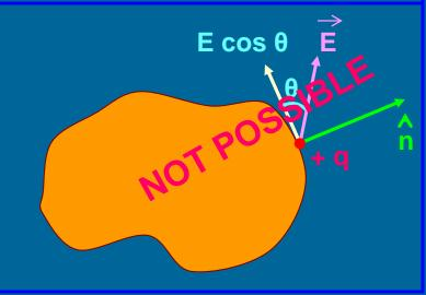
3. Net charge in the interior of a conductor is zero.
