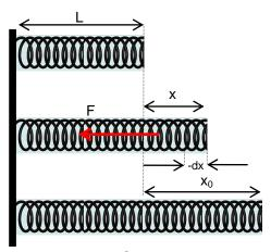
Consider a spring of natural length 'L' & spring constant 'k' its length is increased by  $x_o$ . Elastic potential energy of stretched spring will be equal to total work done by the spring in regaining its original length.
