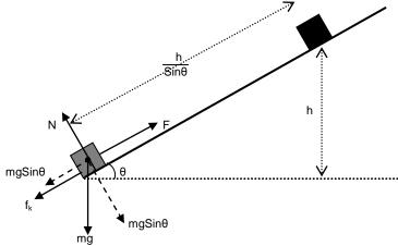
Minimum force required to slide the body up the rough inclined plane having coefficient of kinetic friction  $\mu$  with the body is
