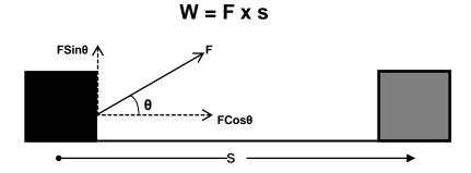
If force and displacement are not parallel to each other rather they are inclined at an angle, then in the evaluation of work component of force (F) in the direction of displacement (s) will be considered.
