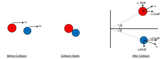
When the centers of mass of two bodies are not along the same straight line, the collision is said to be oblique. In such condition after collision bodies are deflected at some angle with the initial direction. In this type of collision momentum conservation is applied separately along x-axis and y-axis. If the collision is perfectly elastic energy conservation is also applied.
