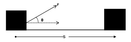
Force and displacement both are vector quantities but their product, work is a scalar quantity, hence work must be scalar product or dot product of force and displacement vector.
