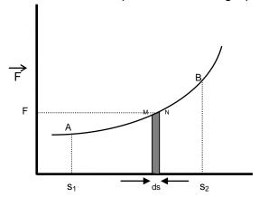
To find work done from  $s_1$  to  $s_2$  we consider two points M & N very close on the graph such that magnitude of force (F) is almost same at both the points. If elementary displacement from M to N is ds, then elementary work done from M to N is.
