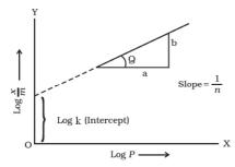
The slope of the line is  $\frac{1}{n}$  and intercept will be equal to log k.
