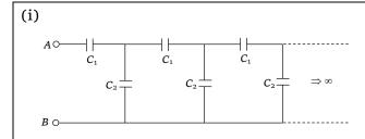
Suppose the effective capacitance between A and B is  $C_R$ . Since the network is infinite, even if we remove one pair of capacitors from the chain, remaining network would still have infinite pair of capacitors, i.e., effective
