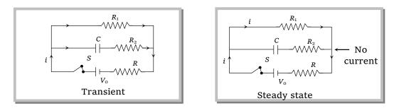
When capacitor gets fully charged (steady state), no current flows through the line in which capacitor is connected. Therefore the current through resistor  $R_1$  is  $\frac{V_0}{(R_1 + r)}$ , hence potential
