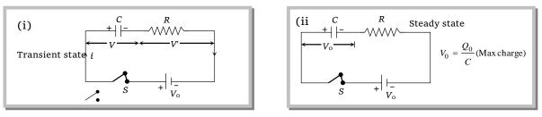
(i) **Charging :** In transient state of charging charge on the capacitor at any instant  $Q = Q_0 \left(1 - e^{\frac{-t}{RC}}\right)$  and potential difference across the capacitor at any instant  $V = V_0 \left(1 - e^{\frac{-t}{RC}}\right)$
