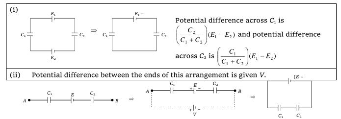
(7) **Advance case of compound dielectrics :** If several dielectric medium filled between the plates of a parallel plate capacitor in different ways as shown.
