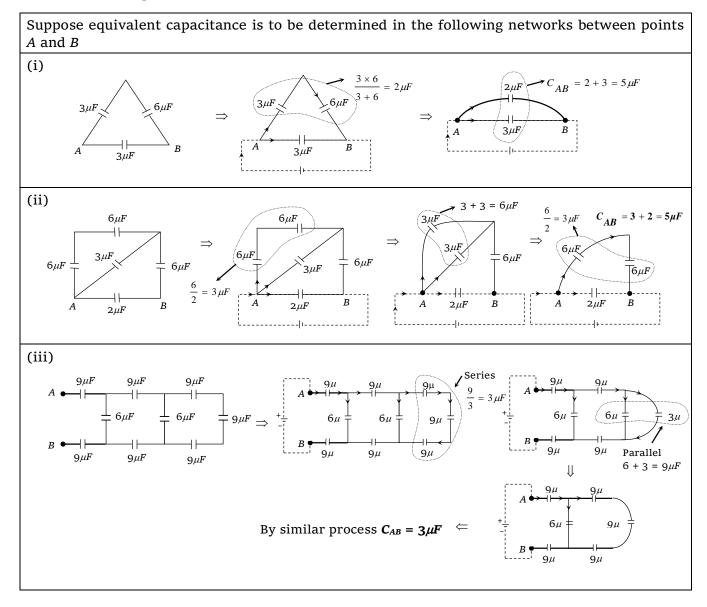
(2) **Circuits with extra wire :** If there is no capacitor in any branch of a network then every point of this branch will be at same potential. Suppose equivalent capacitance is to be determine in following cases
