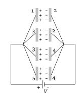
**Example: 143**Four plates are arranged as shown in the diagram. If area of each plate is A and the distance between two neighbouring parallel plates is *d*, then the capacitance of this system between A and B will be
