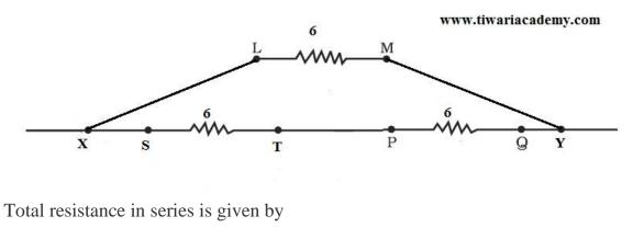
$$R_{12} = R_1 + R_2 = 6 \ \Omega + 6 \ \Omega = 12 \ \Omega$$
