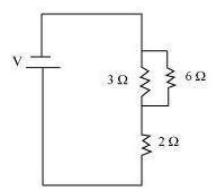
Since, 3  $\Omega$  and 6  $\Omega$  resistors in parallel, so the net resistance
