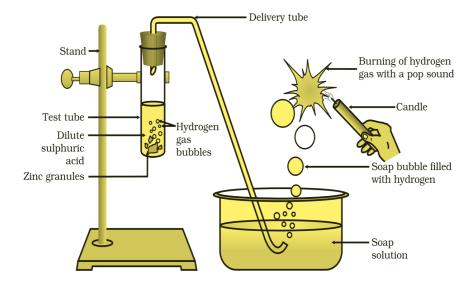
Take few pieces of zinc granules and add 5 ml of dilute H<sub>2</sub>SO<sub>4</sub>. Shake it and pass the gas produced into a soap solution. The bubbles of the soap solution are formed. These soap bubbles contain hydrogen gas.
