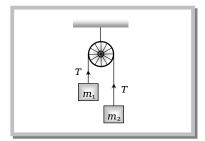
Solution: (b) Tension in the wire  $T = \frac{2m_1m_2}{m_1 + m_2}g$ : stress in the wire  $= \frac{T}{S} = \frac{2m_1m_2g}{S(m_1 + m_2)}g$
