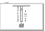
On suspending a weight Mq, the length l of elastic wire and area of cross-section A its Problem 3. length becomes double the initial length. The instantaneous stress action on the wire is
