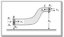
Mathematically for unit volume of liquid flowing through a pipe.
