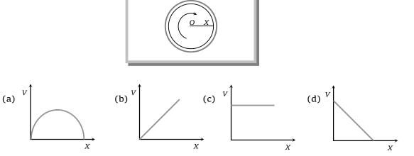
Solution : (d) When we move from the centre to the circumference the velocity of liquid goes on decreasing and finally becomes zero
