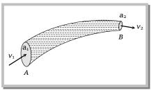
Mass of the liquid entering per second at A = Mass of the liquid leaving per second at B
