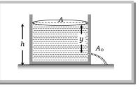
Solution : (b)  $v = \sqrt{2gh} = \sqrt{2 \times 10 \times 20} = 20 \ m/s$
