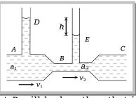
**Problem** 36. In the following fig. is shown the flow of liquid through a horizontal pipe. Three tubes *A*, *B* and *C* are connected to the pipe. The radii of the tubes *A*, *B* and *C* at the junction are respectively 2 *cm*, 1 *cm* and 2 *cm*. It can be said that the
