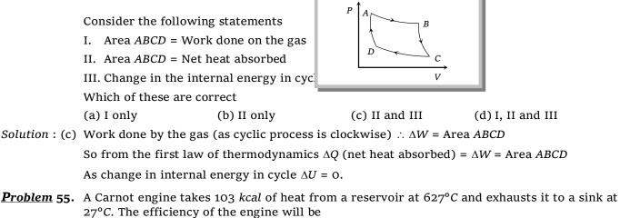
(a) 22.2% (b) 33.3% (c) 44.4% (d) 66.6% Solution : (d) Efficiency of Carnot engine  $=\frac{T_1 - T_2}{T_1} = \frac{900 - 300}{900} = \frac{6}{9}$  or 66.6%.
