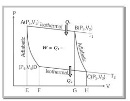
$$W_3 = Q_2 = -\int_{V_3}^{V_4} P \, dV = -RT_2 \log_e \frac{V_4}{V_3} = RT_2 \log_e \frac{V_3}{V_4} = \text{Area } CDFH$$
