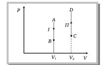
(2) **Indicator diagram :** Graph I and II represent isometric decrease in pressure at volume  $V_1$  and isometric increase in pressure at volume  $V_2$  respectively and slope of indicator dP
