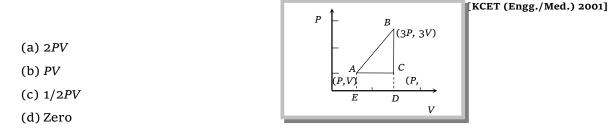
Solution : (a) Work done = Area enclosed by triangle  $ABC = \frac{1}{2}AC \times BC = \frac{1}{2} \times (3V - V) \times (3P - P) = 2PV$
