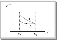
(ii) **Expansion :** If a gas expands isothermally and adiabatically from volume  $V_i$  to  $V_f$  then from the slope of the graph it is clear that graph 1 represent isothermal process, graph 2 represent adiabatic process.
