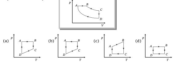
Solution : (a) AB is isobaric process, BC is isothermal process, CD is isometric process and DA is isothermal process
