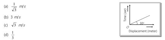
Solution : (c) In first instant you will apply  $v = \tan \theta$  and say,  $v = \tan 30^{\circ} = \frac{1}{\sqrt{3}}$  m/s. But it is wrong because formula  $v = \tan \theta$  is valid when angle is measured with time axis. Here angle is taken from displacement axis. So angle from time axis  $= 90^{\circ} - 30^{\circ} = 60^{\circ}$ . Now  $v = \tan 60^{\circ} = \sqrt{3}$
