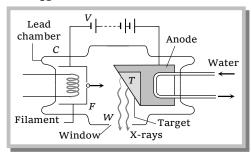
The filament is heated by passing the current through it. A high potential difference ( $\approx$  10 kV to 80 kV) is applied between the target and cathode to accelerate the electrons which are emitted by filament. The stream of highly energetic electrons are focussed on the target.
