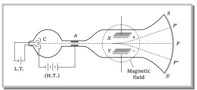
C = Cathode, A = Anode, F = Filament, LT = Battery to heat the filament, V = potential difference to accelerate the electrons, SS' = ZnS coated screen, XY = metallic plates (Electric field produced between them)
