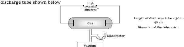
The discharge tube is filled with the gas through which discharge is to be studied. The pressure of the enclosed gas can be reduced with the help of a vacuum pump and it's value is read by manometer.
