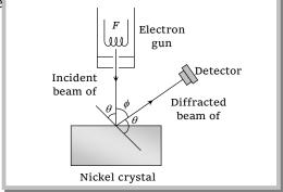
The diffracted beam of electrons is received by the detector which can be positioned at any angle by rotating it about the point of incidence. The energy of the incident beam of electrons can also be varied by changing the applied voltage to the electron gun.
