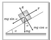
Thus the coefficient of limiting friction is equal to the tangent of angle of repose.
