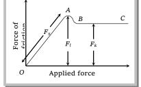
(4) As the portion *BC* of the curve is parallel to *x*-axis therefore kinetic friction does not change with the applied force, it remains constant, whatever be the applied force.
