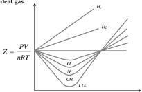
(4) It is difficult to determine quantitatively the deviation of a real gas from ideal gas behaviour from the P-V isotherm curve as shown above. Compressibility factor Z defined by the equation,
