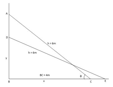
So it is given that foot of the ladder is pulled along the ground away from the wall, at the rate of 0.5m/sec
