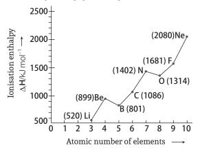
**Ans.** There is deviation of ionisation enthalpy of some elements from the general trend as shown in figure. The first ionisation enthalpy of B is lower than that of Be and in case of nitrogen, the first ionisation enthalpy is higher than that of O. (*Also, refer to Q.* 27)
