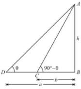
Given that: angle of elevation of top of the tower are  $\angle D = \theta$  and  $\angle C = 90^{\circ} - \theta$ . Distance BC = b and BD = a Here, we have to find the height of tower.
