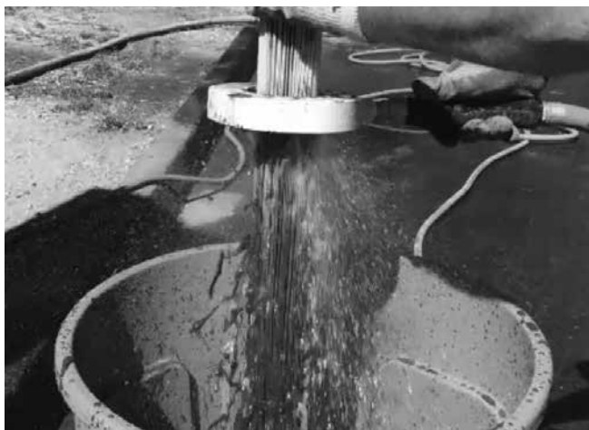
Rinsing Cartridge with Contech Rinse Tool
