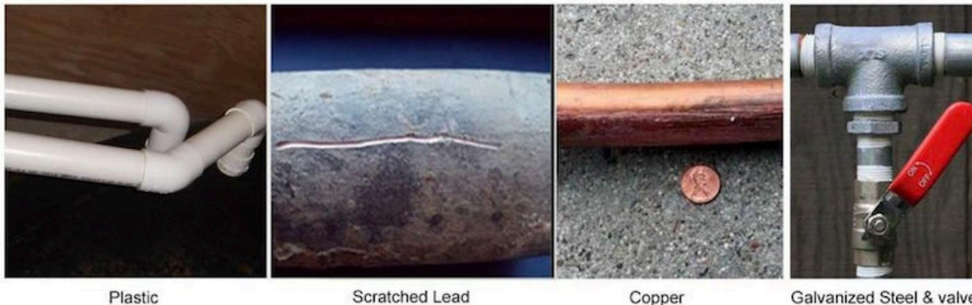
**Plastic:** This pipe comes in different materials and colors. If you tap it with a coin, the pipe does not make a ringing sound.
