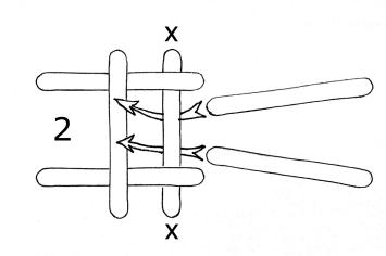
2) Raise the foundation structure by lifting the cross-piece from the ends (marked with "X" on this diagram). You might need someone to help you do this. Once you've lifted it, slide two sticks under the cross-piece and OVER the other cross-piece. It is okay for them to overlap more than they do in this picture. When the sticks are in place, lower the cross-piece that you've lifted and allow the force of gravity to lock the bridge pieces into place.
