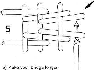
by repeating steps 3 & 4 as many times as you can! 4) Lift the newest cross-piece to elevate one end of the bridge and then slide in two additional span sticks (just like you did in step two) to make the span of your bridge even longer. Lower the cross-piece to allow gravity to lock the pieces into place.
