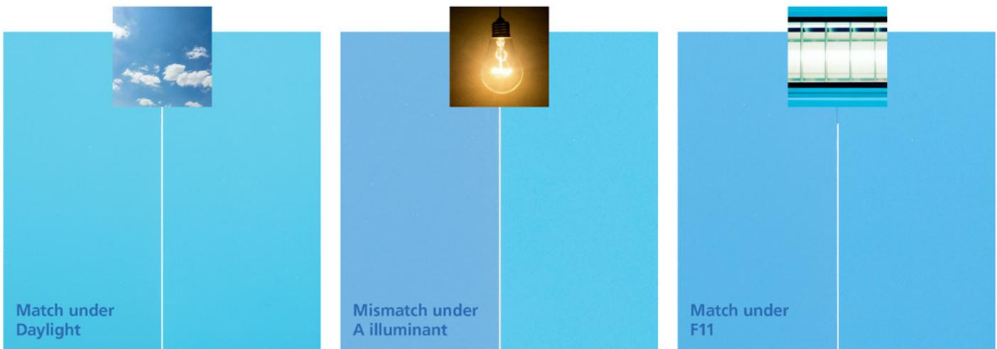
Graphic courtesy of BYK Gardner - Depending on the application, color needs to match under a variety of illuminants. This is particularly important for multi-component products consisting of different materials
