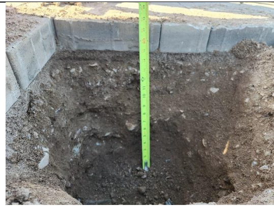
TP-1 - The subgrade is similar to the AB except the subgrade has rocks as large as three inches
