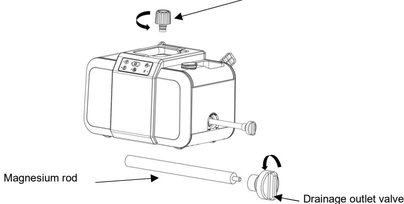
3. Follow descaling agent instructions to fill up descaling agent into boiler, leave it for 30-60 minutes. Unscrew drain outlet valve, empty boiler.
