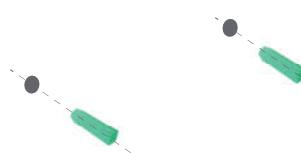
5. Insert the screws through the holes in the wall bracket and tighten them securely using a screwdriver, ensuring they are locked into the screw anchors. Installation is complete.
