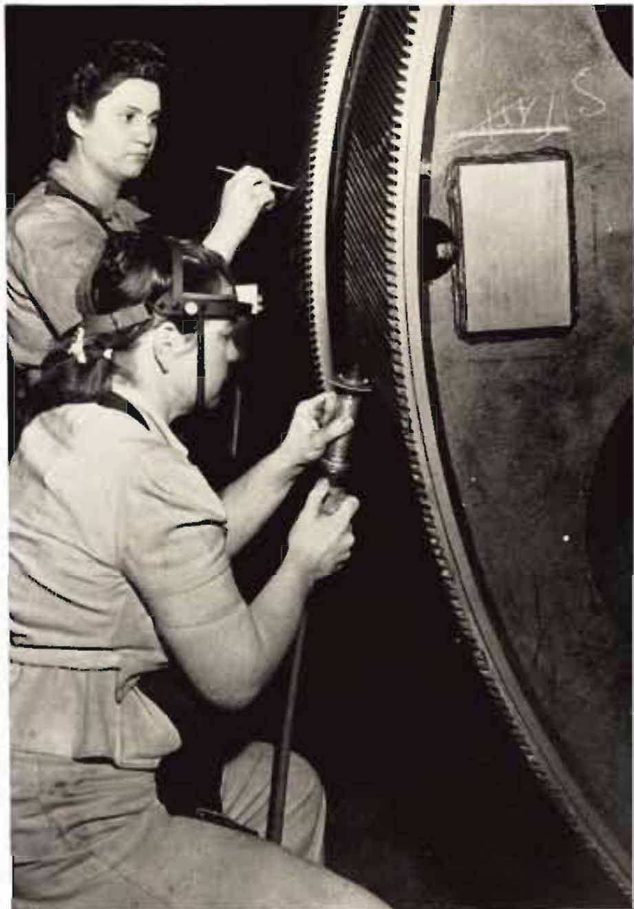
Tolerance on the reduction gears of the Hendy turbine is kept at a minimum of .0002, necessitating exacting finishing work, a large part of which is performed by women workers.
