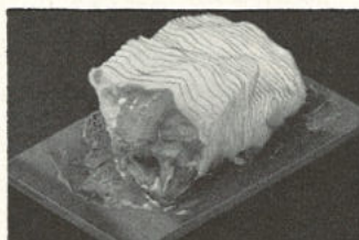
Wafers of precise thickness and parallelism are sliced from mother quartz with Di-Met Rimlock diamond abrasive wheels.
