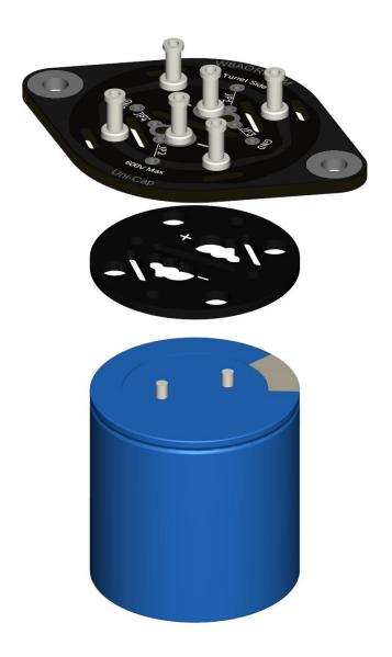
This kit is designed to replace single, high voltage can capacitors with 46 mm CTC mounting hole spacing. These cans were frequently used in old audio and radio frequency equipment and are typically 1-3/8 to 1-9/16 inches in diameter.
