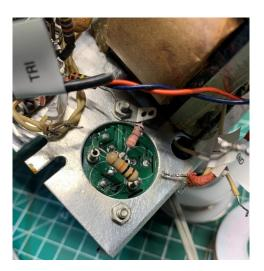
14. Connect the associated cables and resistors to the proper locations. I usually start with the Transformer Center Tap to Ground lead first with the 330k ohm resistor (replace with new-optional) that goes to pin 2 of V1 (12AX7).
