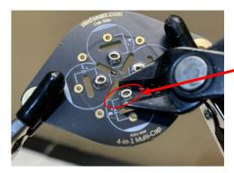
Slightly squeeze the short end of the Solder Post Turret on the "Cap Side". It requires very little pressure.
