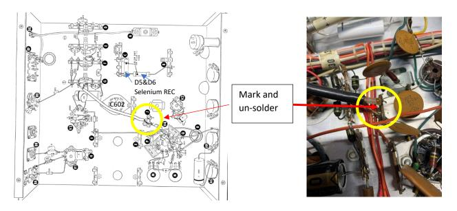
7. Note the orientation of the 4 sections of the Multi-Sectional Can Capacitor. On the bottom of the capacitor there will be three cut outs, Half Moon, Triangle and Square. The 4<sup>th</sup> one is sometimes marked with a Dash or left blank. The top and bottom of the supplied Multi-Cap board will also be marked with Half-Moon, Triangle, Square and Dash. The Heathkit Manual does not depict this very well. The orientation is as marked below. May be installed 180' from diagram.
