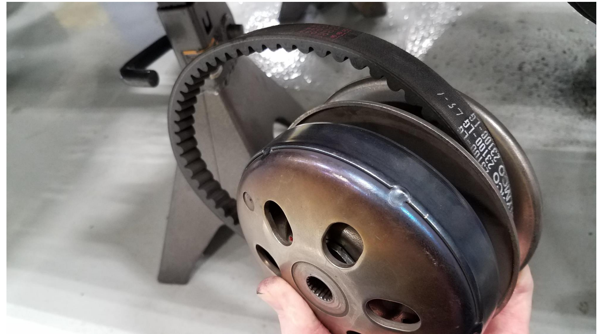
The belt and driven clutch are removed as a set.
