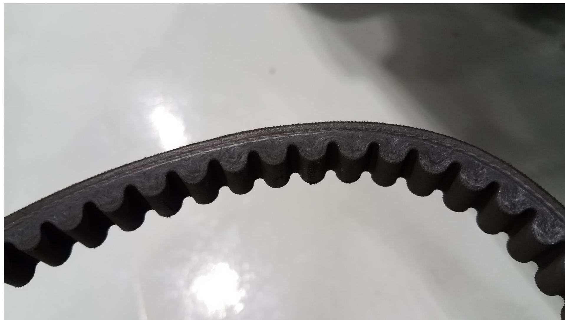
Inspect the belt for glazing, cracking, fraying, and separation. Replace the belt if necessary.
