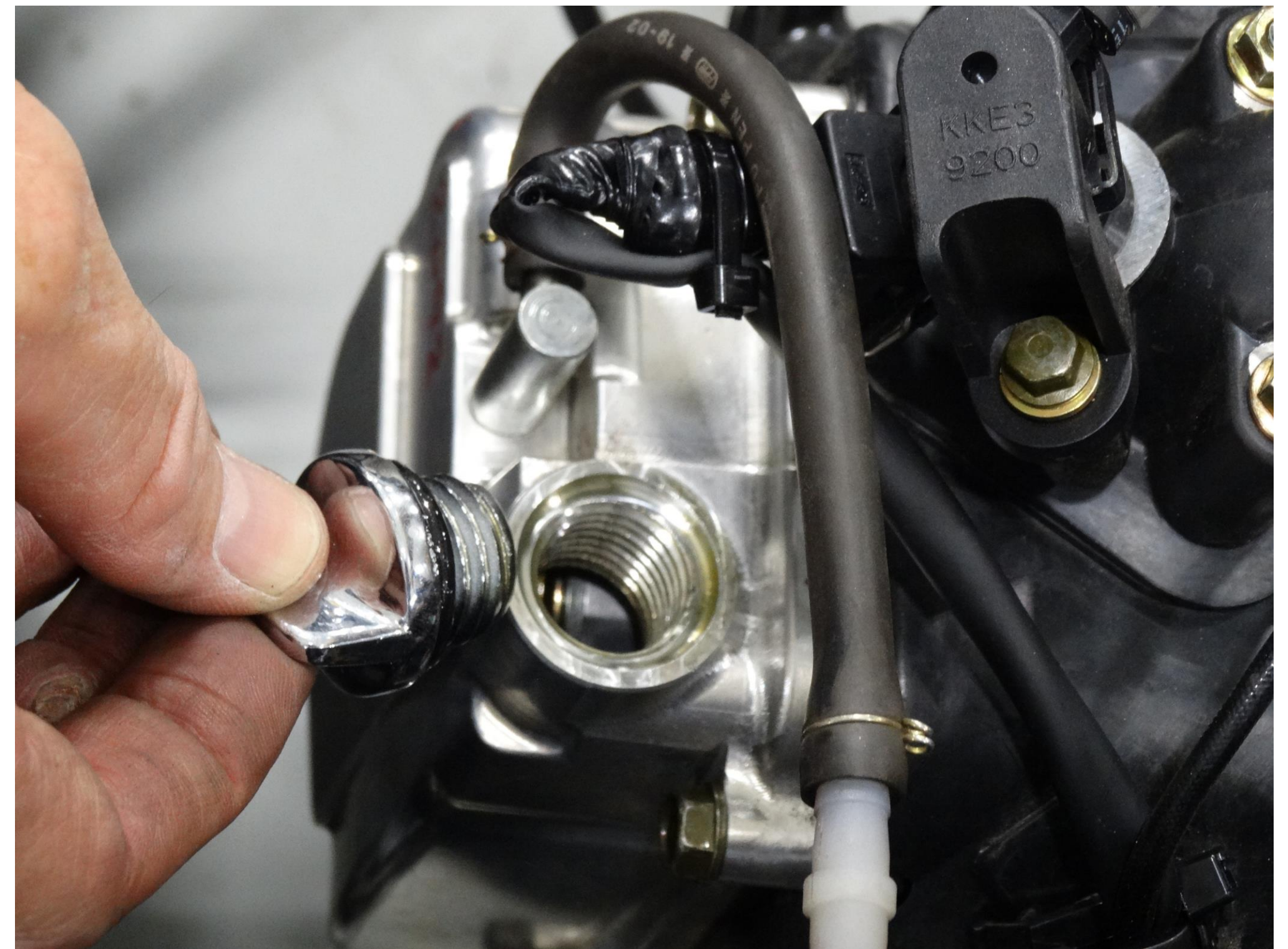
The oil level is adjusted through the plug on the top of the valve cover.
