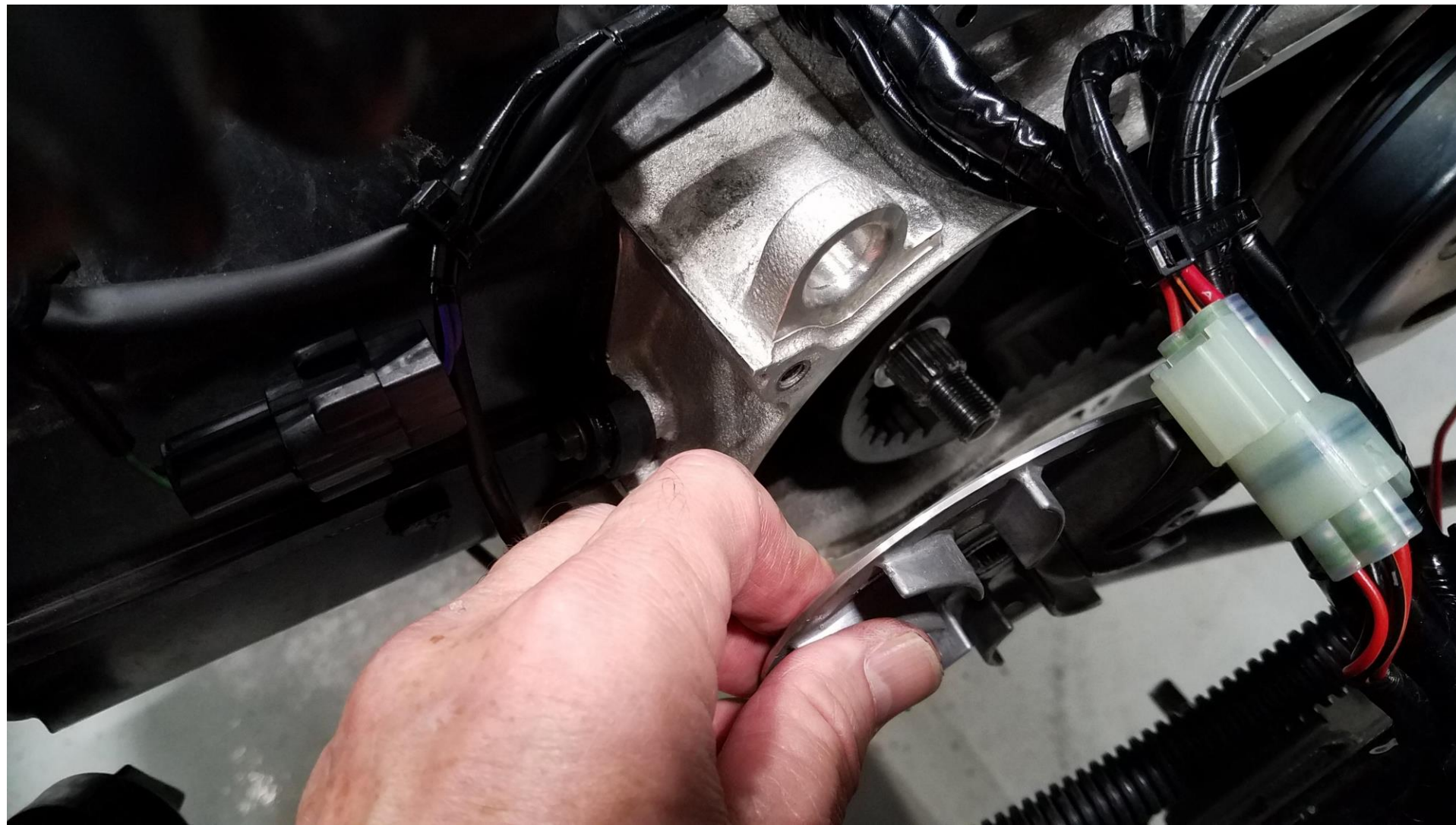
Remove the drive clutch outer sheave.
