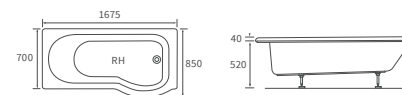
ORA 1700MM P SHAPE SHOWER BATH LH AND RH Overall height including screen 2055mm. Capacity 200 litres
