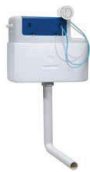
Apex Cistern - Side Inlet 446(w) x 363(h) x 133(d)mm 3/4 Litre Flush Side entry inlet valve Top or front flush plate mounting 1/2 BSP, PS Insulation jacket, pneumatic flush valve with chrome flush button Cistern
