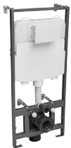
1170mm Wall Hung WC Frame with Front Operated Cistern 800(w) x 1148(h) x 140-200(d)mm 3/4 Litre Flush Use for In-wall applications Requires flush plate/bush or contactless sensor 200mm height adjustment Frame & Cistern
