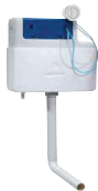
Vortex Cistern - Bottom Inlet 434(w) x 343(h) x 133(d)mm 3/4 Litre Flush Bottom entry inlet valve Top or front flush plate mounting 1/2 BSP, PS Insulation jacket, pneumatic flush valve with chrome flush button Cistern
