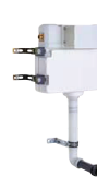
In-Wall Cistern 400(w) x 294(h) x 138-194(d)mm 3/4 Litre Flush Ideal for fixed applications All parts accessible through flush plate aperture 150mm height adjustment Internal bottom entry valve Top or front flush plate mounting 1/2 BSP, PS Insulation jacket Cistern
