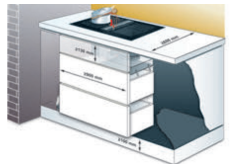
The cut-out dimensions for flush installation are W = 780/804 mm x D = 500/524 mm; please take stepped cut-out into consideration. The cutout dimensions for surface-mounted installation (with or without a frame) W = 780 mm x D = 500 mm.
