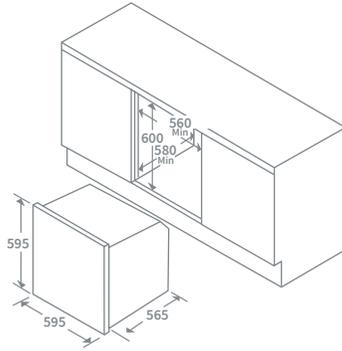
**BUILT-IN SINGLE ELECTRIC FAN OVEN**
