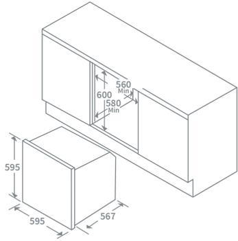
**BUILT-IN SINGLE ELECTRIC FAN OVEN**
