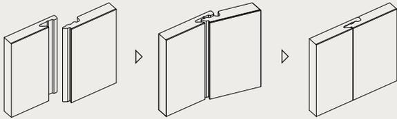
**Sureseal** is a four point sealing system that achieves greater sealing performance at the base of the Showerwall Laminate panel. Fit and forget using the only maintenance free shower seal on the market with no future resealing required.
