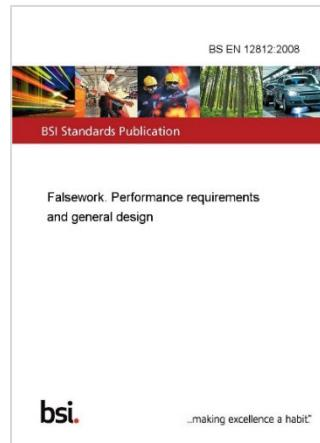
**BS EN 12812** covers falsework design over 3 metres (**BS5975 Section 3** covers the falsework design up to 3 metres)
