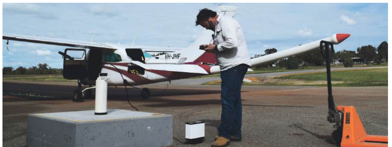
Photo: A geophysical survey technician undertakes calibration work on Thomson Airborne's Cessna 210M at Northam airfield
