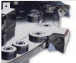
5. 3 DECK MOUNTED TEETH & RECUTTER BAR FOR A FINER FINISH
