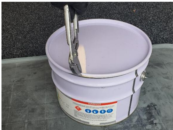
Remove the lid carefully and allow gasses to vent. Use pliers to carefully lift the edge of the lid.
