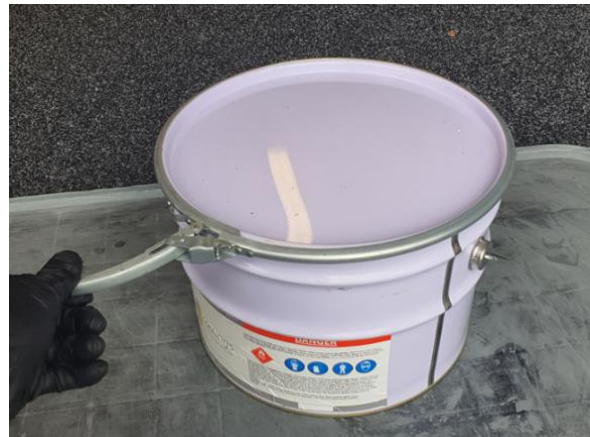
Remove ring seal – Be careful when removing the seal as gasses might pop the lid. Remove the lid carefully and allow gasses to vent.
