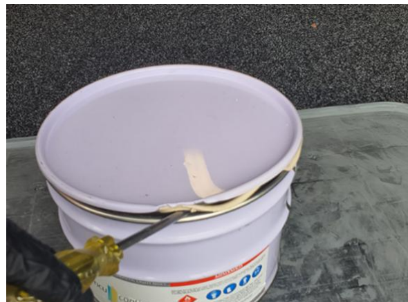
Use a sharp object such as a screwdriver and knock it between the can rim /lid & lift the lid upwards.
