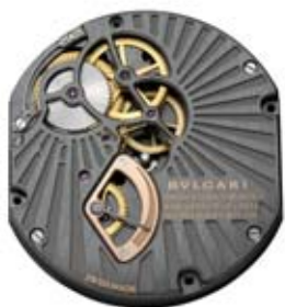
BVL 266 CALIBER MANUFACTURE CALIBER WITH FLYING CENTRAL TOURBILLON AND PATENTED PAPILLON FUNCTION Mechanical movement with manual winding, flying central tourbillon, Papillon Minutes indication system and jumping hours. Caliber decorated by hand with perlage, fine sandblasting and golden engraving on its visible back-side. 60-hour power reserve.
